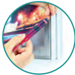
Attach graphic into SEG frame channel
